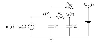
$$C\frac{dT(t)}{dt} = \frac{T_m(t) - T(t)}{R_m} + \frac{T_{out}(t) - T(t)}{R_{out}} + q_c(t) + q_e(t)$$
